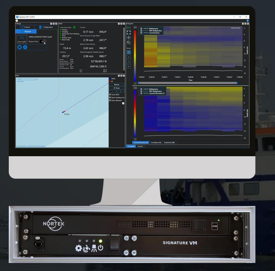
Then we need data acquisition software that allows us to easily discover the instruments, stores the data and just shows that everythings works. The software also drives the LEDs so that you can see statuses at a glance.
